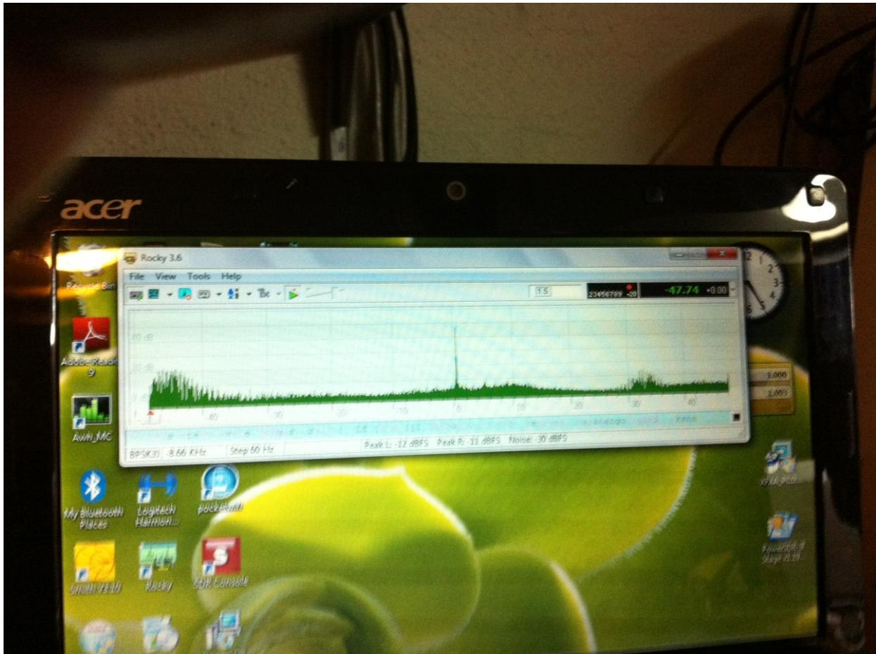
This is a picture of a typical spectrum. Sorry that the picture is a little fuzzy. The centre spike is the usual SDR 0 Hz spike and you can see that the spectrum is about 100kHz. The big lump on the left is QRM and at +35kHz is a signal. You can see more typical spectrums on the site where you downloaded Rocky.
