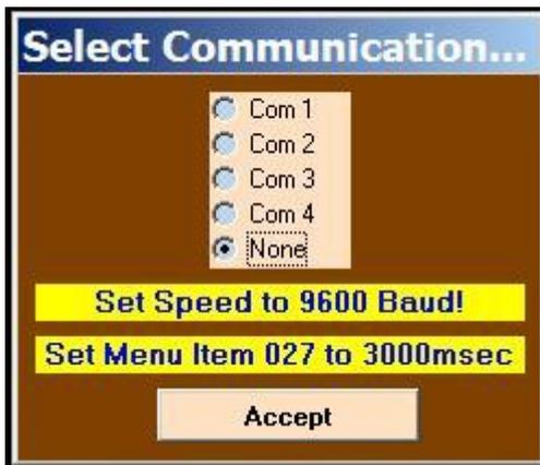
You must now choose which serial communications port to use on your computer. This will correspond to the serial port you identified during the prerequisite instructions that you have your serial cable connected to from the computer to the CAT serial port on your FT-950 rig.
