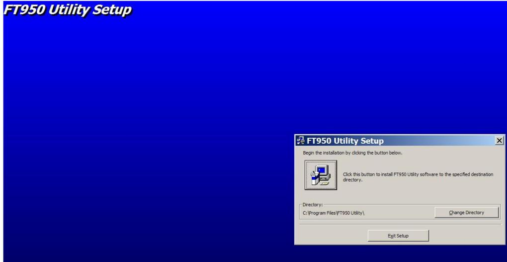
Step 4: You will see the screen shown above - You may accept the current installation location or change the installation directory. It is recommended that you accept the installation directory without change. So just click on the box with computer in it to accept the shown installation directory and begin the installation.
