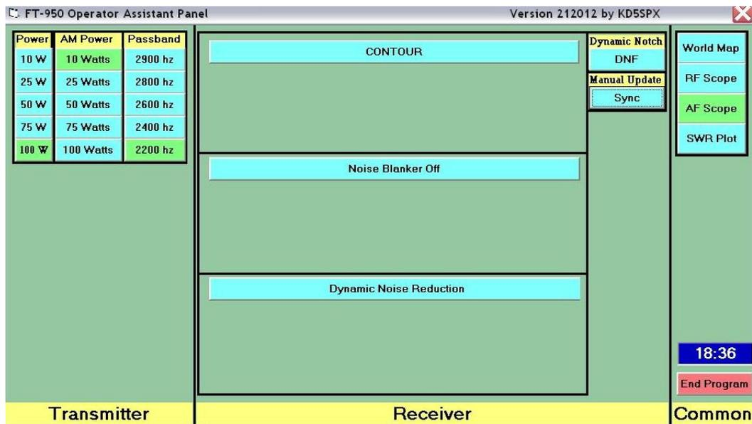
The software after confirming the FT-950 identity and DMU availability then detects the current settings from the FT-950 for the current band and receiver options controlled from the software program. Buttons on the screen which are illuminated green indicate the current settings read from your FT-950 for functions controlled by this software utility program.
